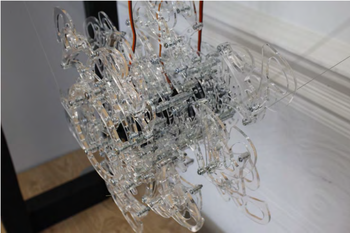
Figure 74 The mechanical design of The Flower of Time V.2 was an assemblage of four mechanical layers. The first layer on the left was the layer of second, then from left to right, the layer of minute, hour and day
