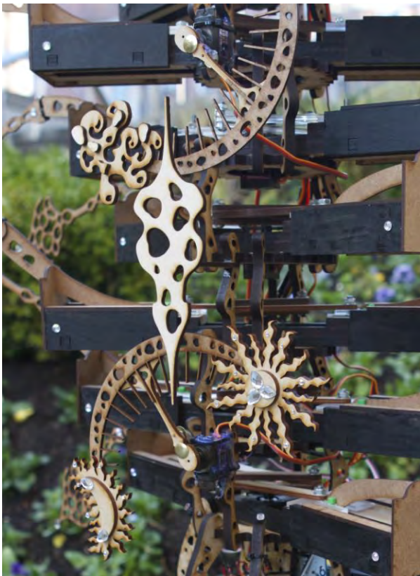
Figure 63 A meter showing the soil humidity (top) and light quantity (bottom) on Botanical Clock . For the light quantity meter, the shape of sun indicated bright environment while the shape of moon indicated dark environment
